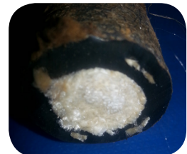
Load bearing fibres protected by thick, black rubber skin
